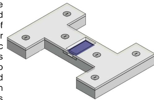
**Figure 4: Chip-holder design for GaAs thin film waveguides.**
