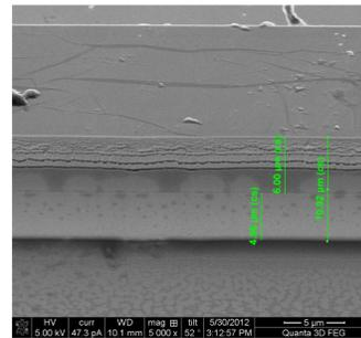
After spincoating a photoresist onto the surface, the wafer was exposed to UV radiation via a manual mask aligner. The subsequent development process lead to photoresist MZI patterns, which were then transferred to the wafer via RIE.
